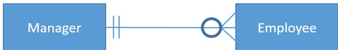
Fig N: An example of a mixed relationship. A manager can manage none, one or many employees, but one or one or many employees have to report to a manager. Note the two vertical lines next to the 'Manager' entity to show 'one and only one', and the circle next to the 'crow's foot' to show the 'zero or many' optionality of the mixed relationship.
